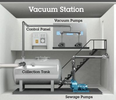
Our completely closed vacuum sewer collection system prevents infiltration and inflow of groundwater from the valve pit to the vacuum station, protecting waterways from exfiltrating wastewater.
