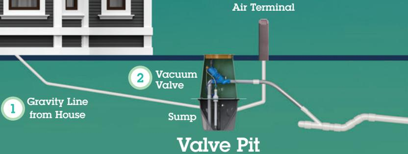
**1** A traditional **gravity line** carries wastewater from the customer to an Airvac **valve pit**.
