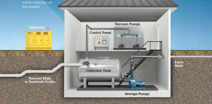
Our completely closed vacuum sewer collection system prevents infiltration and inflow of groundwater from the valve pit to the vacuum station, protecting waterways from exfiltrating wastewater.
