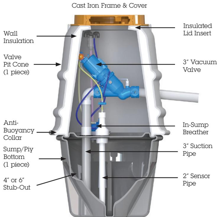
All other pit components (sump/pit bottom, sensor pipe, in-sump breather, suction pipe, anti-buoyancy collar, etc.) are identical to those included with the standard 2-piece valve pit.
