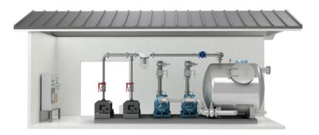
PacVac Version 1 includes a 1-story, at-grade or partially buried prefabricated building that houses all the mechanical equipment on 1 level. All the mechanical equipment is assembled on 1 skid and is supplied by Airvac. The prefabricated building is supplied by Airvac.
