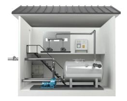
PacVac Version 2 contains similar equipment as PacVac Version 1 but rather than everything on a single level, the equipment is arranged in an over/under configuration in a two-story structure.
