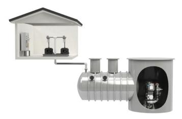
PacVac Version 3 utilizes a direct-bury fiberglass collection tank to eliminate the need for a basement. Dry pit submersible sewage pumps are housed in either an adjacent inexpensive operator friendly vault or in a fiberglass structure that is fabricated as part of the collection tank itself (shown above). The vacuum pumps and control panel are in a prefabricated building supplied by Airvac.
